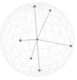
The state of the pendulum is entirely determined by the position of the bob. The bob can move from any point at a fixed distance (equal to the length of the rod) from the centre to any other. The configuration space is therefore a two-dimensional sphere, and the spherical pendulum has two degrees of freedom.
