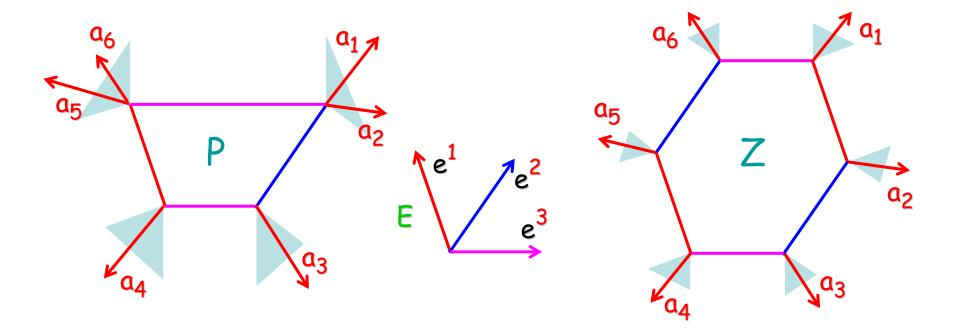
Lemma: In R<sup>d</sup>, the zonotope Z can be constructed from E = { $e^1$ , ...,  $e^m$ } along with a vector  $a_i$  in the cone of every vertex in  $O(m^{d-1})$  operations. (Edelsbrunner, Gritzmann, Orourk, Seidel, Sharir, Sturmfels, ...)
