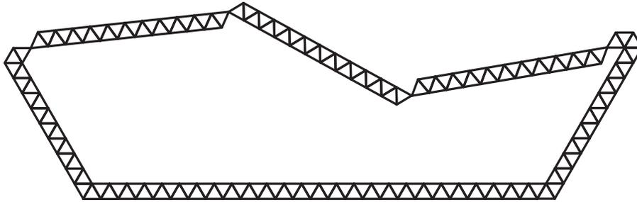
When the base is held fixed there is one degree of freedom in these configurations, and they form a stratum of  $\overline{\mathbb{E}P}(n)$  homeomorphic to a circle. More generally, with  $k$  trusses whose total length is slightly longer than the distance between the support points at the ends of the base, the stratum is homeomorphic to a sphere  $S^{k-2}$ . This can be seen by induction on  $k$ , each increase in  $k$  producing a suspension of the previous space of configurations.
