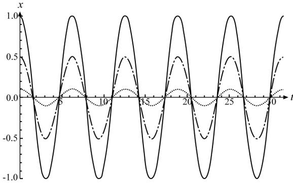
**FIGURE 2.** Numerically obtained time responses of the equation of motion (36), i.e. (46), for different initial conditions,  $\dot{x}(0)=0$  and:  $x(0)=1$  (solid line),  $x(0)=0.5$  (dashed line) and  $x(0)=0.1$  (dotted line).
