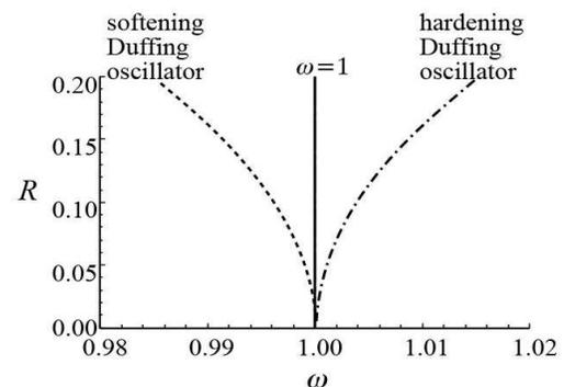
**FIGURE 1.** Numerically obtained backbone curves of the Duffing oscillator (2) (dotted and dashed-dotted lines) and a straight-line backbone curve (solid line).
