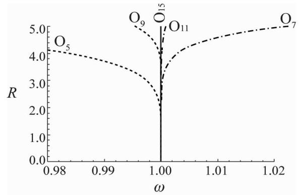
**FIGURE 3.** Numerically obtained backbone curves of the oscillator (31) with the coefficients defined by Eq. (30) for a different number of odd-powered terms (the highest power is indicated in the subscript).
