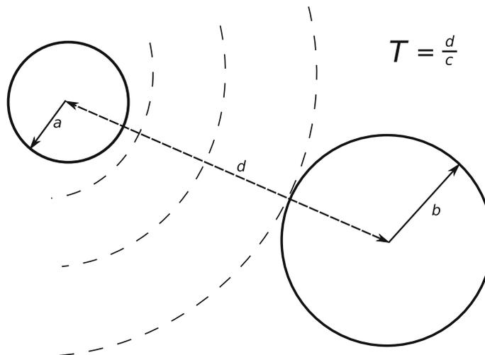
**Fig. 1.** Two bubbles submerged in a liquid. Note that bubble  $b$  also influences bubble  $a$  with an induced acoustic wave. Delay  $T = d/c$  where  $d$  is the distance between bubbles and  $c$  is sound speed.
