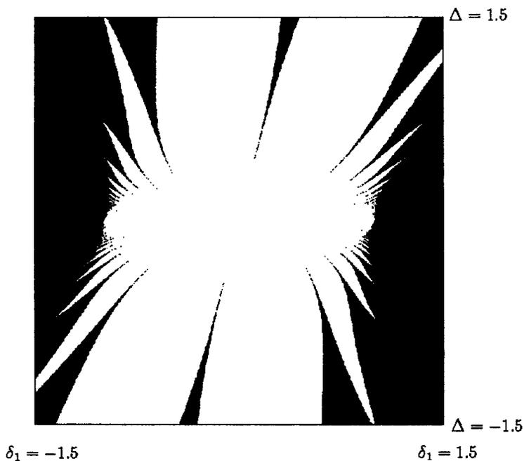
Figure 2. Stability chart obtained by numerically integrating slow flow Equation (9) for  $\mu = 1$ . Points in the blackened regions correspond to absence of limit cycles (stable). Points in the white regions correspond to the presence of limit cycles (unstable). Compare with Figure 1.
