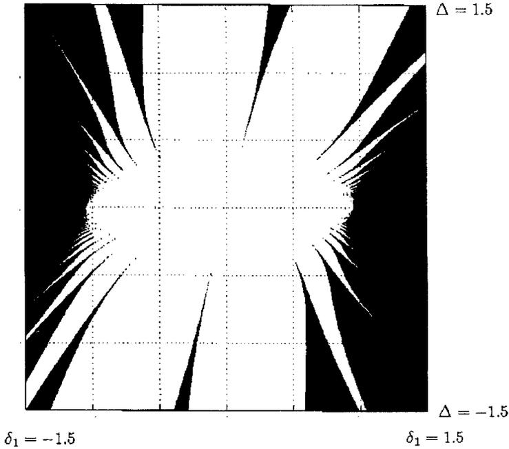
Figure 1. Stability chart of the QP Mathieu equation (1) obtained using numerical integration by Zounes [9] for parameters  $\varepsilon = 0.1$  and  $\mu = 1$ . Here  $\delta = 1/4 + \delta_1 \varepsilon$ . Points in the blackened regions correspond to stable (bounded) motions. Points in the white regions correspond to unstable (unbounded) motions.
