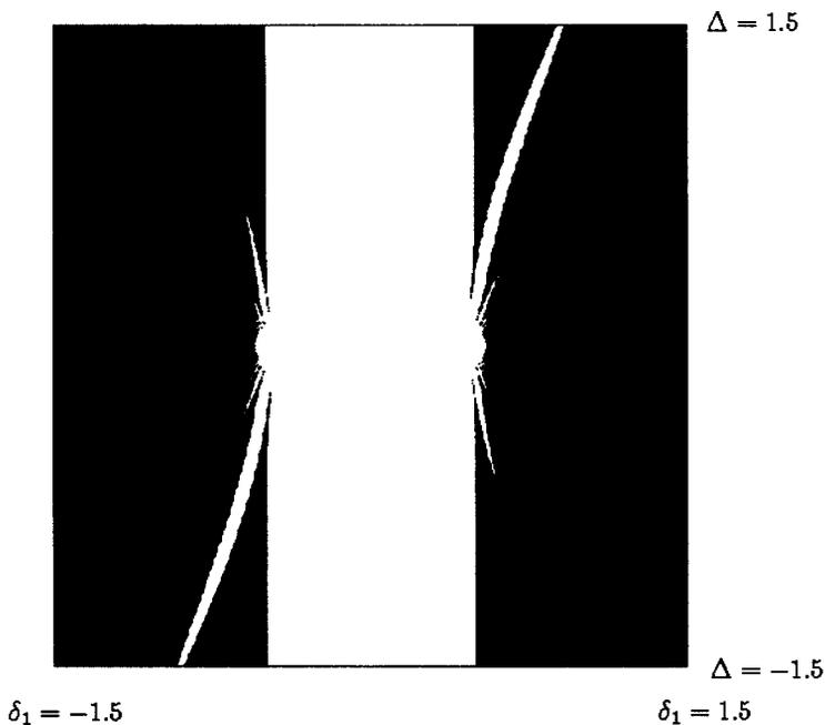
Figure 3. Stability chart obtained by numerically integrating slow flow Equation (9) for  $\mu = 0.1$ . Points in the blackened regions correspond to absence of limit cycles (stable). Points in the white regions correspond to the presence of limit cycles (unstable).
