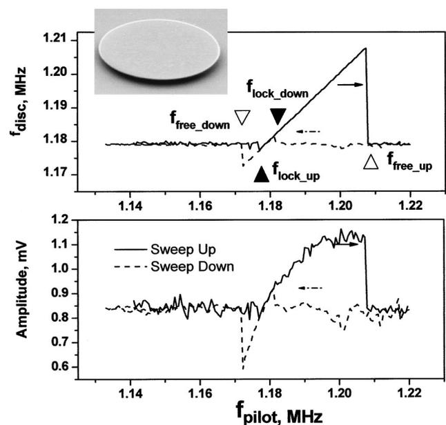
FIG. 1. Frequency and amplitude of the laser-induced self-sustained vibrations as a function of the pilot signal frequency. Laser power  $P_{\text{cw}} = 650 \mu\text{W}$ , perturbation applied as an inertial drive ( $V_{\text{piezo}}^{\text{ac}} = 4 \text{ Vol}$ ).
