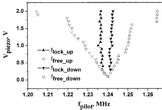
FIG. 2. Entrainment zone as a function of the pilot signal amplitude. Laser power  $P_{cw} = 1.7$  mW, perturbation applied as an inertial drive. A discontinuity in the width of the entrainment zone at  $V_{piezo} \sim 1.8$  V is observed when the expanded entrainment zone overlaps the areas that allow different types of limit-cycle oscillations.
