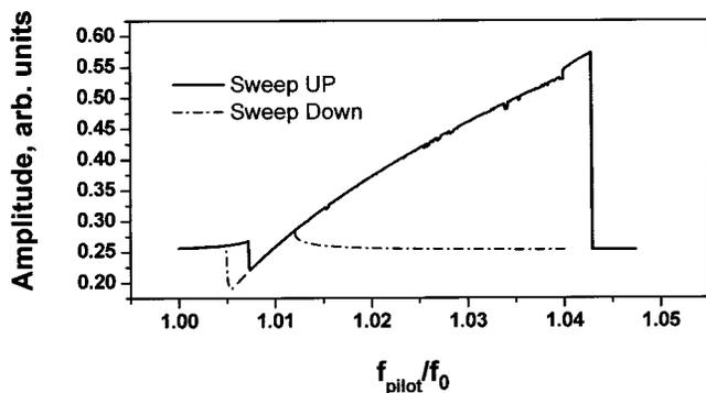
FIG. 4. Result of numerical simulations for the amplitude of the laser-induced self-sustained vibrations as a function of the inertial drive pilot signal frequency ( $P_{cw}=650 \mu\text{W}$ ). The amplitude of inertial drive  $M=10^{-4}$ , modulation  $\varphi$  in Eq. (2) has been taken as zero.
