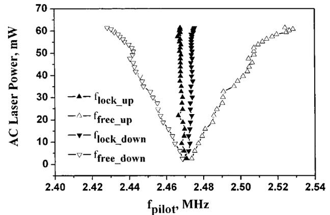
FIG. 3. Entrainment zone as a function of the pilot signal power. Laser power  $P_{cw} = 1.7$  mW, perturbation applied as a modulation of the secondary laser beam (Ar+) positioned at the center of the disk.
