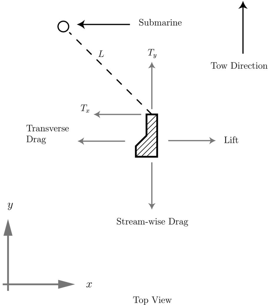
Figure 1: Free body diagram of submarine towing a plate. Figure is in a horizontal plane.
