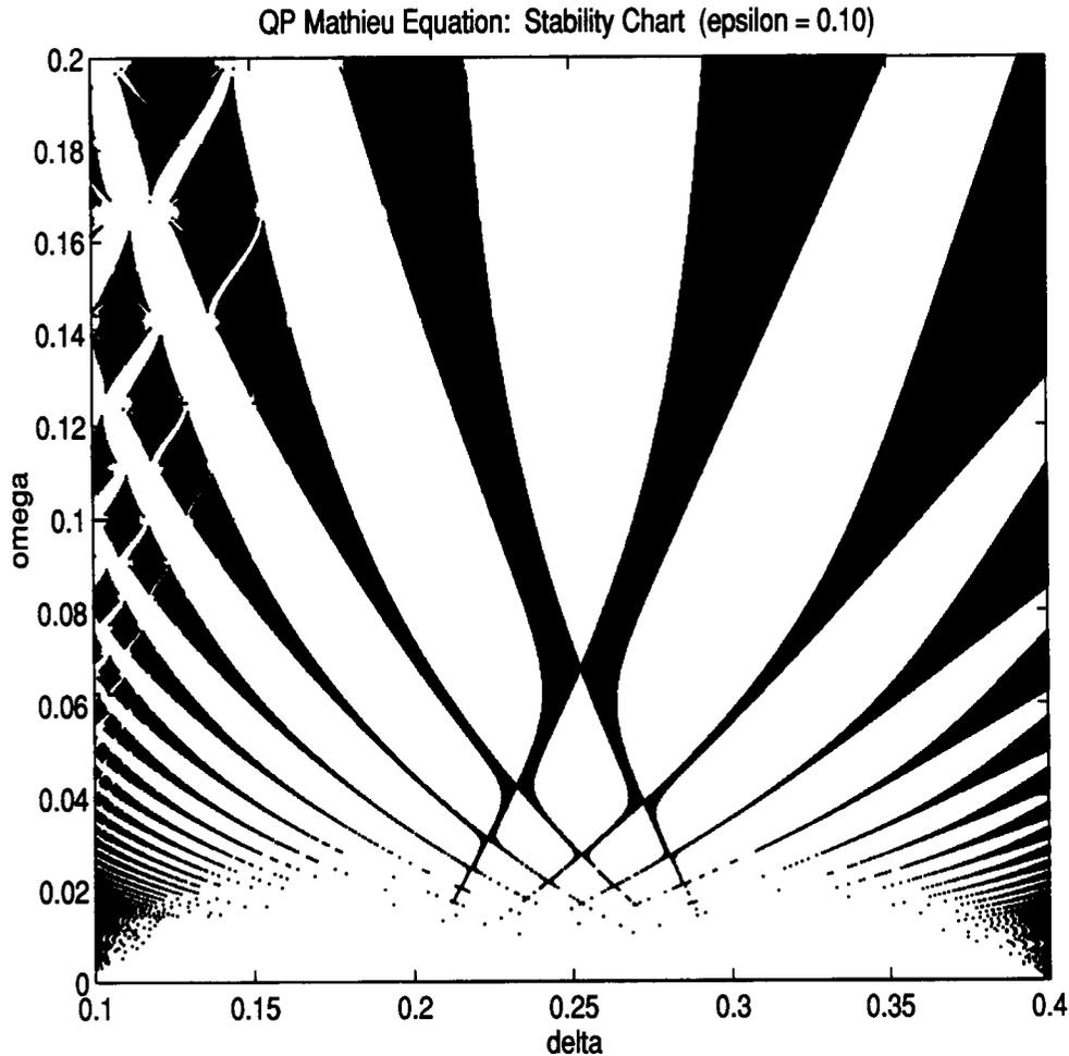
FIG. 2.2. Stability chart of the QP Mathieu equation generated from numerical integration utilizing the second procedure. Points  $(\delta, \omega)$  in the blackened regions of the  $\delta$ - $\omega$  parameter plane correspond to bounded (stable) solutions.
