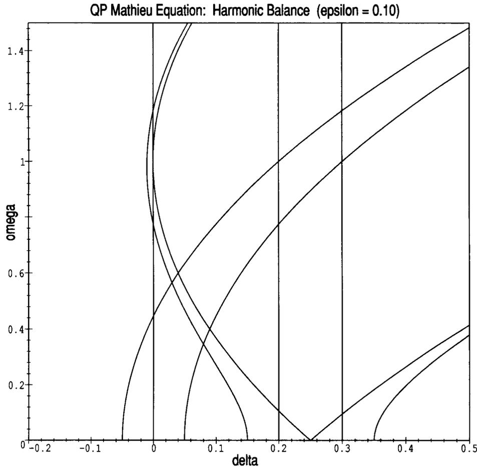
FIG. 5.1. Transition curves for the QP Mathieu equation (1.1) as determined by the method of harmonic balance,  $\epsilon = 0.10$ . Truncation order:  $N = 1$ .
