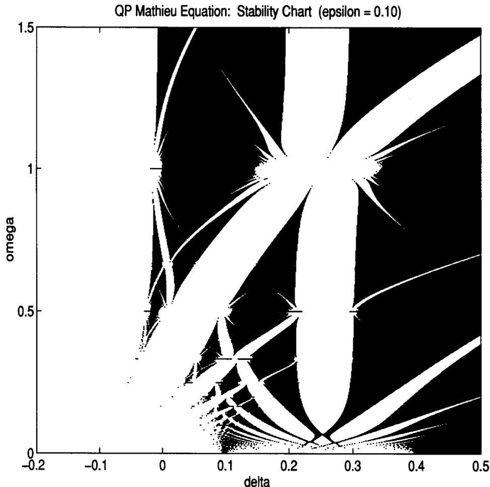
FIG. 2.1. Stability chart of the QP Mathieu equation generated from numerical integration utilizing the first procedure:  $T_{\max} = 20000$ ,  $R = 10^6$ , and  $\epsilon = 0.10$ . Points  $(\delta, \omega)$  in the blackened regions of the  $\delta$ - $\omega$  parameter plane correspond to bounded (stable) solutions.
