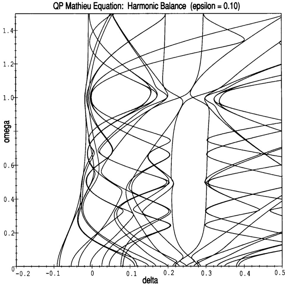
FIG. 5.2. Transition curves for the QP Mathieu equation (1.1) as determined by the method of harmonic balance,  $\epsilon = 0.10$ . Truncation order:  $N = 4$ .
