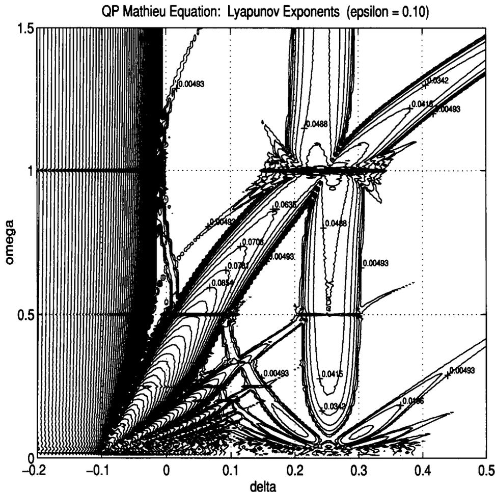
FIG. 3.1. Contour plot of Lyapunov exponents associated with the QP Mathieu equation. The level curves correspond to constant values of  $\lambda > 0$  on which unbounded solutions of equation (1.1) exist.
