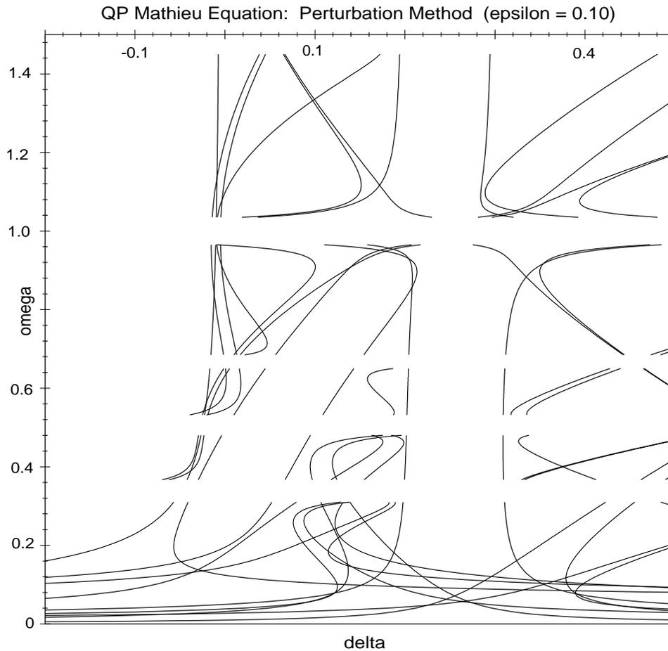
FIG. 4.1. Transition curves for the QP Mathieu equation (1.1) as determined by the perturbation method,  $\epsilon = 0.10$ . The regions around resonant values of  $\omega$  have been omitted.
