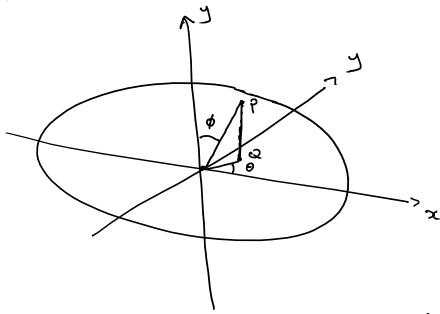
P = point on ellipsoid Q = projection of P to xy-plane
