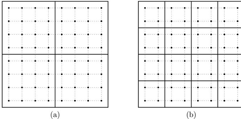
FIG. 2. Two examples with different domain decompositions. Both (a) and (b) are based on the same grid (dotted), with  $M = 8^2$  and  $h = 1/7$ . Figure (a) uses the cell size  $h^c = 4/7$ , the total number of cells  $J = 2^2$ , and  $r = 4$  gridpoints per cell side. Figure (b) uses  $h^c = 2/7$ ,  $J = 4^2$ , and  $r = 2$ .
