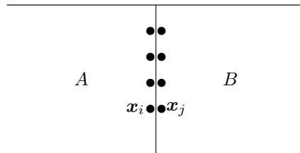
FIG. 3. Suppose that as a result of processing the cell  $A$  an eastern border value  $V_i$  becomes updated. If  $V_i < V_j$  and  $\mathbf{x}_j \notin Q'$ , then cell  $B$  is downwind of cell  $A$ . In this case cell  $B$  will be added onto  $L$  unless already there, its value will be updated, and its preferred sweeping directions will be updated.
