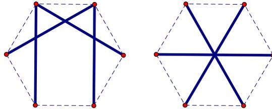
Solution: The following shows how to add a sequence of tensegrities, with a PSD stress to the left one to get the one on the right. At each stage scale the positive cable stresses to cancel with the negative strut stresses, using the symmetry. "Most" small perturbations of the right tensegrity will not have any equilibrium stress.
