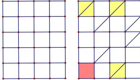
Figure 1: This is a bar framework of  $a = 5$  rows of squares, and  $b = 4$  columns of squares. The framework on the right has  $c = 8$  of the squares braced with diagonal bars.
