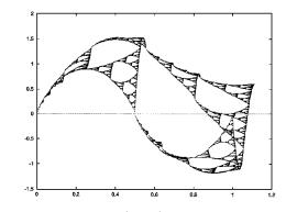
Differential Equations (FDE) on the Sierpinski Gasket (SG). For the first time, computer generated images of solutions to FDEs were produced. The figure shows the graph of an eigenfunction of the Laplacian the fractal analog of the sine function. Other images, including a "movie" of the fundamental solution of the wave equation on SG, are available (http://www.tc .cornell.edu/Edu/SPUR/SPUR96/Kyal/cover.html).
