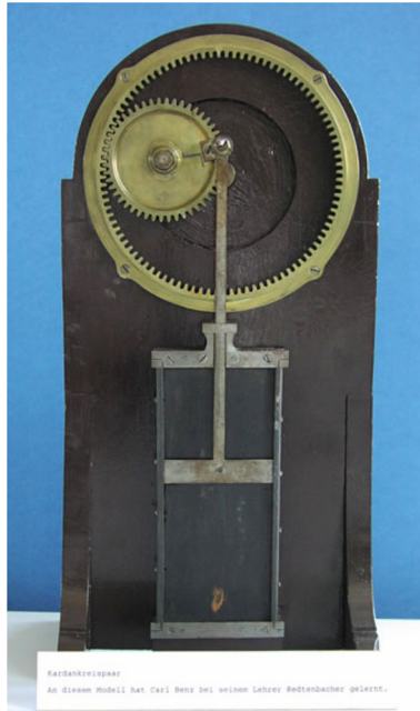
Fig. 2 A mechanism at Cornell, where the point on the inner geared circular wheel traces out a straight line
