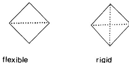
FIG. 8. The solid lines are rods, the dotted lines cables.  $n = 2$ .
