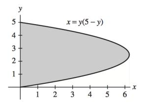
Now suppose the region is rotated about the y-axis. Because a horizontal slice is perpendicular to the y-axis, we will calculate the volume of the resulting solid using the disk method. Each cross section is a disk of radius R = y(5 - y), so the volume is
