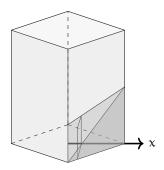
SOLUTION: If we place the center of the base at the origin, then the vertical cross section at a given x will be a rectangle of height x, since the 45 degree plane has equation x = z.
