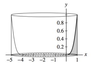
Each shell has radius x - (-2) = x + 2 and height  $x^3$ , so the volume of this solid is
