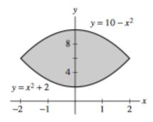
When this is rotated about the x-axis, each cross section is a washer with outer radius  $R = 10 - x^2$  and inner radius  $r = x^2 + 2$ . The volume of the solid of revolution is then
