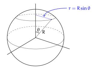
SOLUTION: Because  $r = R \sin \theta$ ,  $dr = R \cos(\theta) d\theta$ . For r to vary between 0 and R,  $\theta$  must vary from 0 to  $\pi/2$ . Substituting into the previous integral, we obtain
