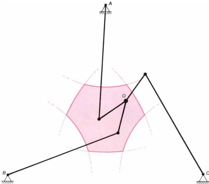
**LINKAGE of three double cranks joined by a central pin also gives rise to a two-manifold. The motion is confined to a plane, and the central pin can reach any point inside the hexagon.**
