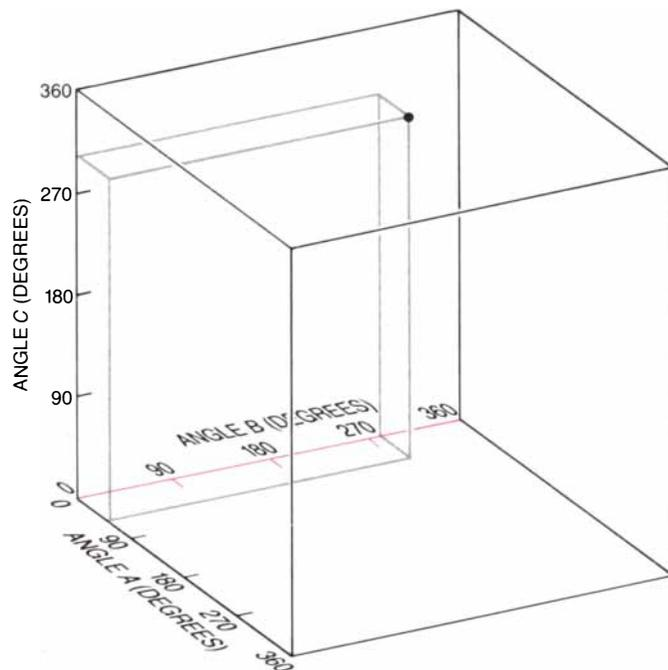
**THREE-MANIFOLD** analogous to the two-torus arises from the set of all possible configurations of a triple crank whose motion is confined to a plane (*left*). If the angles between each bar and a fixed direction are plotted on three mutually perpendicular axes, every possible position of the triple crank can be plotted as a point in a cube
